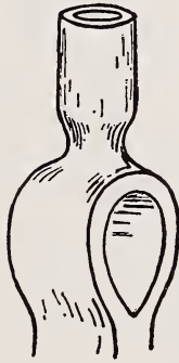
E. the eye is drifted to shape
