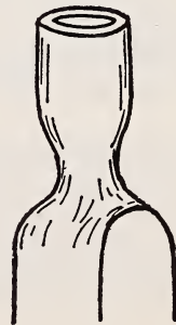
FIGURE 15. The pierced eye technique
