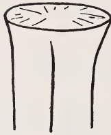
A. the bar of iron at start and after upsetting
