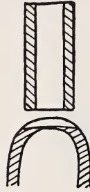
B. tube ready for welding
