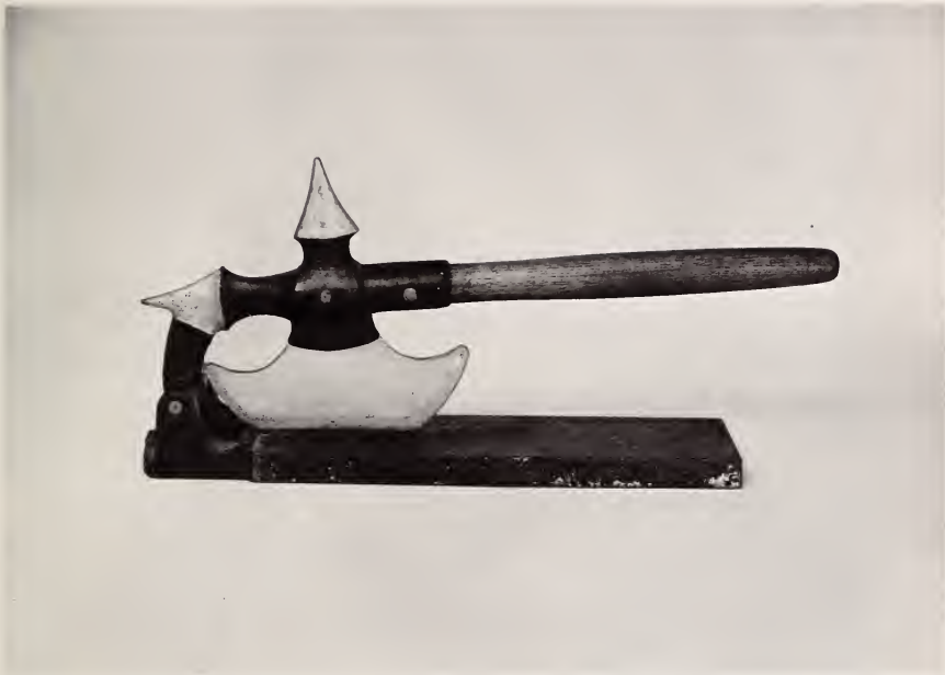
PLUG CUTTER FOR BATTLE AX PLUG TOBACCO, LATE 19TH CENTURY. HEADS BROKEN FROM PLUG CUTTERS SUCH AS THIS ARE OFTEN MISTAKEN FOR TOMAHAWKS OR EARLY POLEARMS. L: 17" MAI/HF: 23/2231
