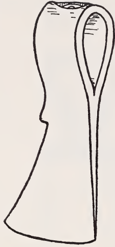
A. blade with forged pocket
